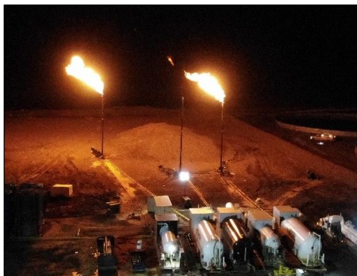
Figure One – Gas Flaring from both horizontal wells during production testing: Calima-2 (left) and Calima-3 (right).
